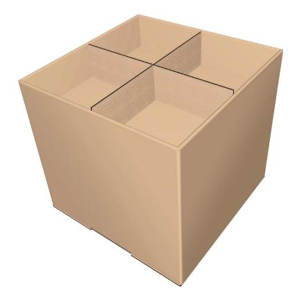
Note: The outer wall is creased at 180 degrees to form a double wall.
